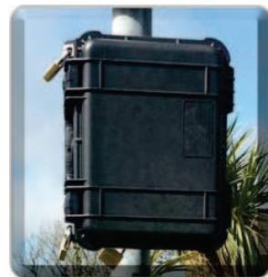
**Nº of Observations:** The number of readings recorded by the radar. This does not correspond to an exact count of vehicles passing the sign, since vehicles may pass the sign in a tightly packed group (or 'platoon'); the radar will only record data for the 'lead vehicle' that is determining the speed for the remainder of the platoon.
